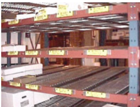
Figure 4 – Gravity Fed Racking
